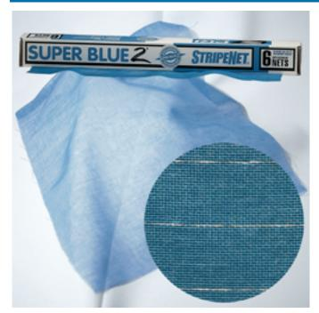
SUPER BLUE 2® StripeNets® anti-marking, antistatic nets are chemically treated non-stretchable, wrinkle-free fabric, which eliminates any maintenance of the net. A soft metallic fiber woven into the net at regular intervals are conductive which helps reduce static electricity build up between printing units. These lines also serve as guides enabling an easy and trouble-free installation process.
