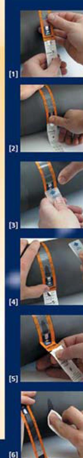
Since the volume of the indicator fluid is constant in all Capatch strips, the length of the track measures the ink volume of the anilox roll cells.
